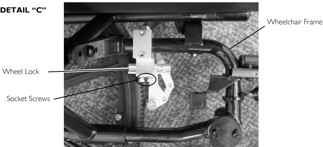
FIGURE 9.2 Adjusting Patient-Operated Wheel Locks
